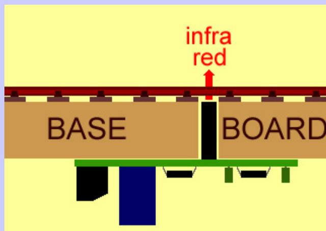
Where it is difficult to fit the detector due to baseboards thicker than 22mm or cross beams under the baseboard the units can be supplied with the infrared emitter and detector connected to the board with wires. These boards are distinguished from standard ones by having EW added on the end (EW stands for Extended Wire).
