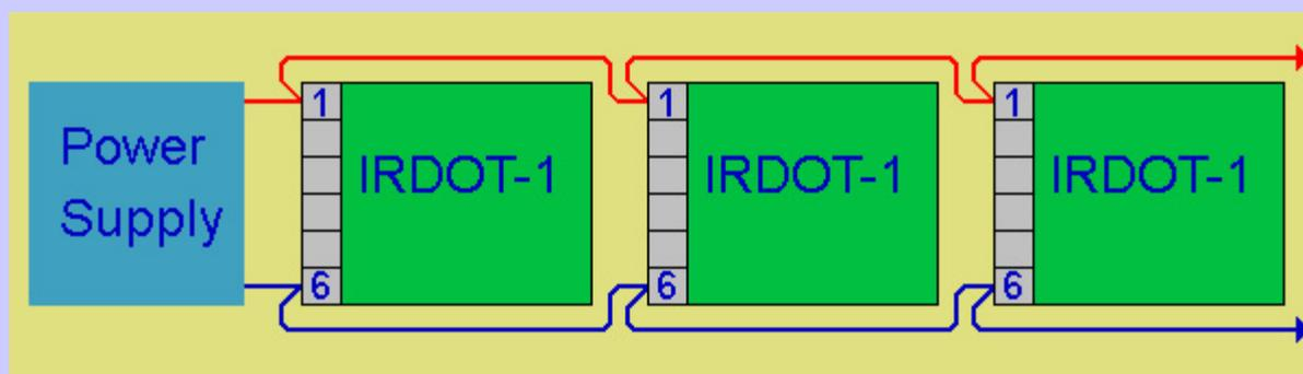
The IRDOT-1 is used to activate other units when it detects a train. Terminal 2 will trigger the Dual Timer, IRDASCs, latching relay board, alternate route selector and SA units. This is described in the pages about these boards.
