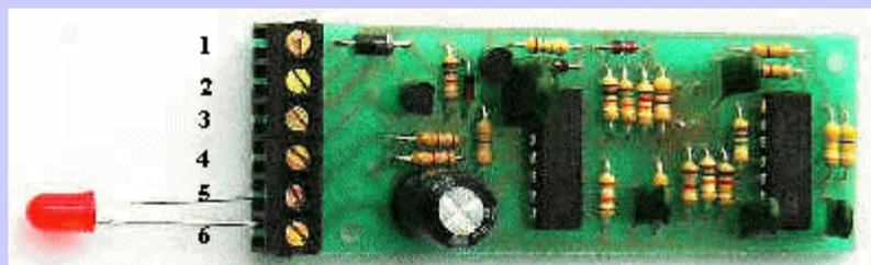
The IRDOT-1 is also used to automatically trigger some of our other boards when the train has reached a certain location. Examples are the SA series of boards Timer, Simple Shuttle, IRDASC-1, 2, 3 and DSS. An advantage over
